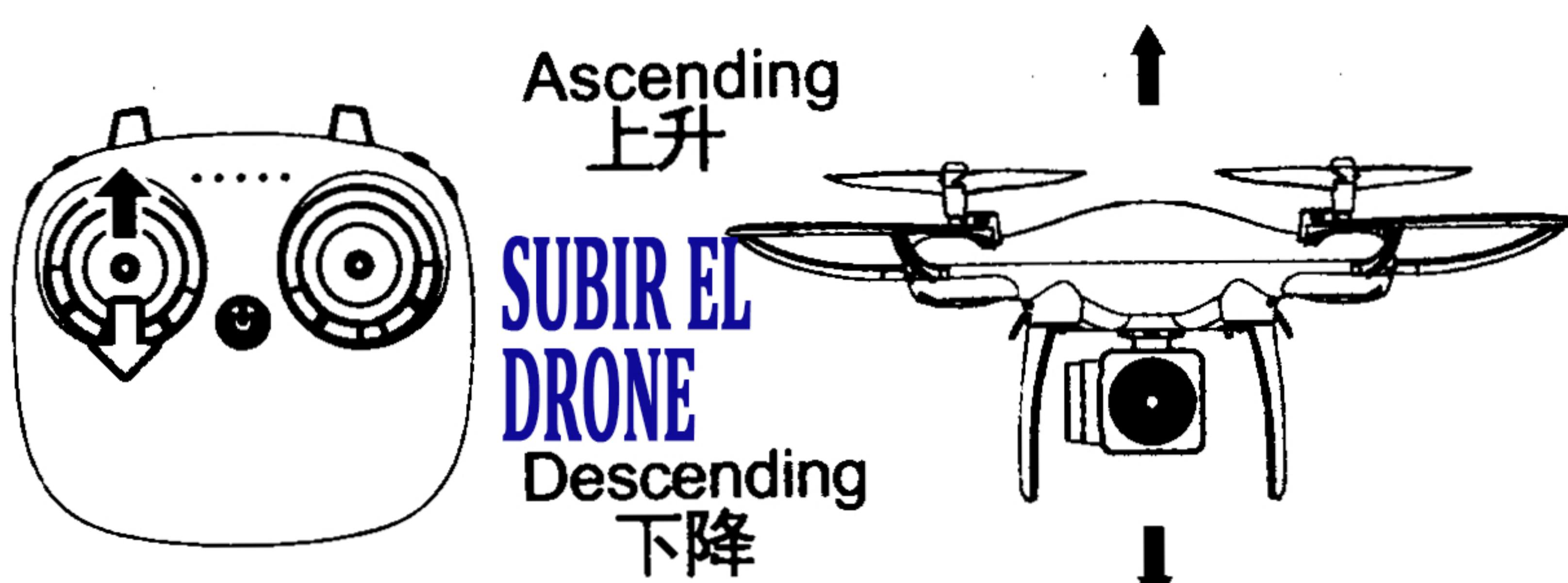
Push up the throttle stick, and the spinning speed of the main blades will increase. The aerocraft begins to ascend.
